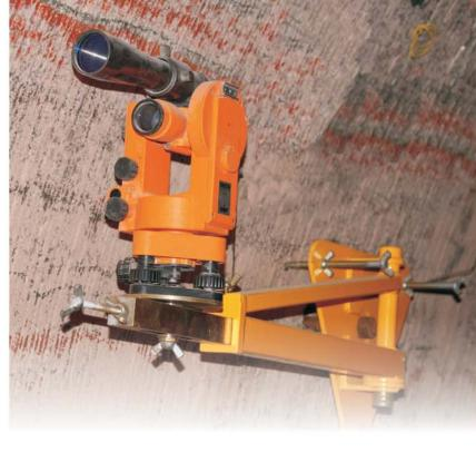
LASER ALIGNMENT SYSTEM CAN BE MOUNTED ON THE ARM FIXED TO WORKING WALL OR GEODETIC
